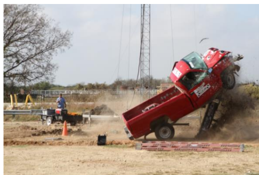
Figure 29. Pickup truck impact test and simulation with LS-DYNA.
