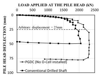
Figure 20. Load settlement curve for conventional and post grouted shafts (after King et al., 2015).
