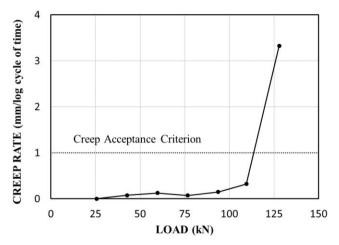
Figure 23. Creep rate for nail NS1 (after Sanchez et al., 2017).
