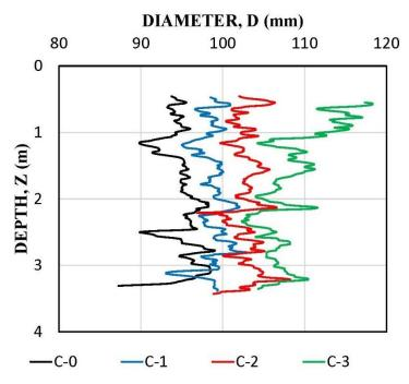
Figure 6. Borehole Erosion Test results (after Briaud et al., 2017).
