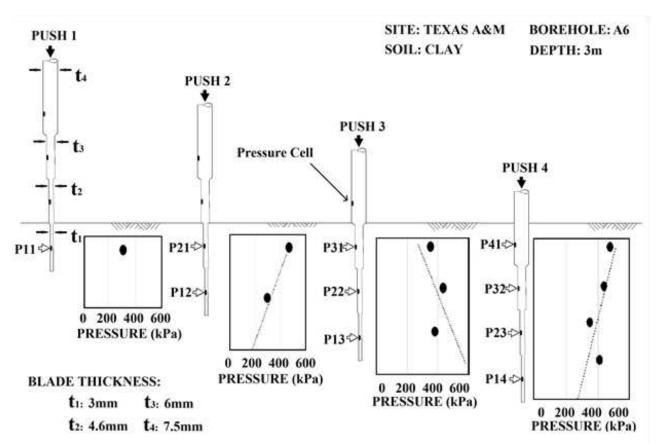
Figure 4. Stepped blade test (after Gan, Briaud, 1987).
