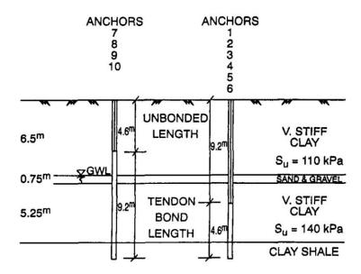
Figure 14. Configuration of the 10 anchors tested (Powers, Briaud, 1993).
