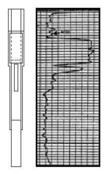
Figure 13. Gamma ray log: a) North quadrant, b) East quadrant (after Briaud, Dupin, 1990).
