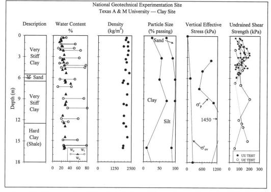
Figure 2. Laboratory test results (Briaud, 1997(a)).
