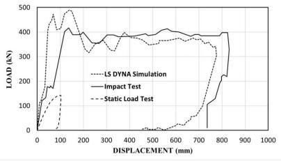
Figure 30. Pile static load and impact load vs. displacement curve.
