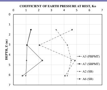
Figure 5. Coefficient of earth pressure at rest from prebored pressuremeter (PBPMT), self-boring pressuremeter (SBPMT), and stepped blade (SB) (after Gan, Briaud, 1987).
