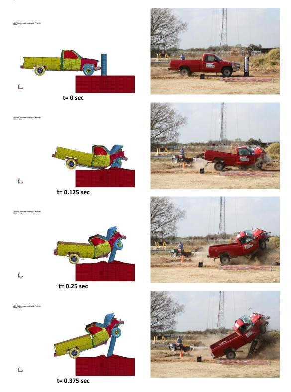
Figure 29. Pickup truck impact test and simulation with LS-DYNA.
