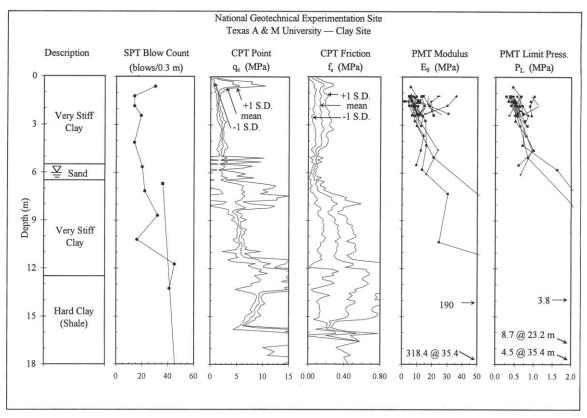
Figure 3. In-situ test results (Briaud, 1997(a)).
