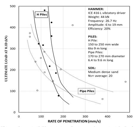
Figure 29. Ultimate pile capacity (D/10 criterion) vs. vibration rate of penetration (after Bossher et al., 1998).
