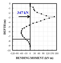
Figure 22. Wall bending moment profile at end of construction for one row of anchors (after Chung, Briaud, 1992).
