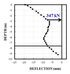
Figure 21. Wall deflection profile at end of construction for one row of anchors (after Chung, Briaud, 1992).
