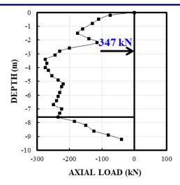
Figure 23. Wall vertical load at end of construction for one row of anchors (after Chung, Briaud, 1992).
