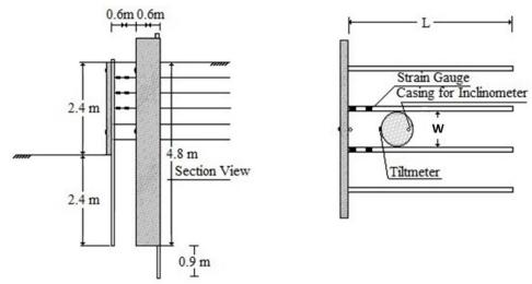
Figure 31. Setup and dimensions.
