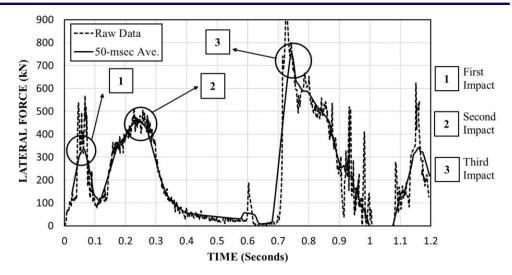
Figure 35. Impact load on the barrier during the event from numerical simulation.
