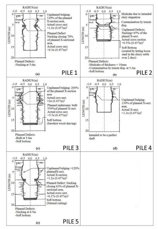
Figure 12. Five drilled shafts with planned defects (after Ballouz et al., 1991).
