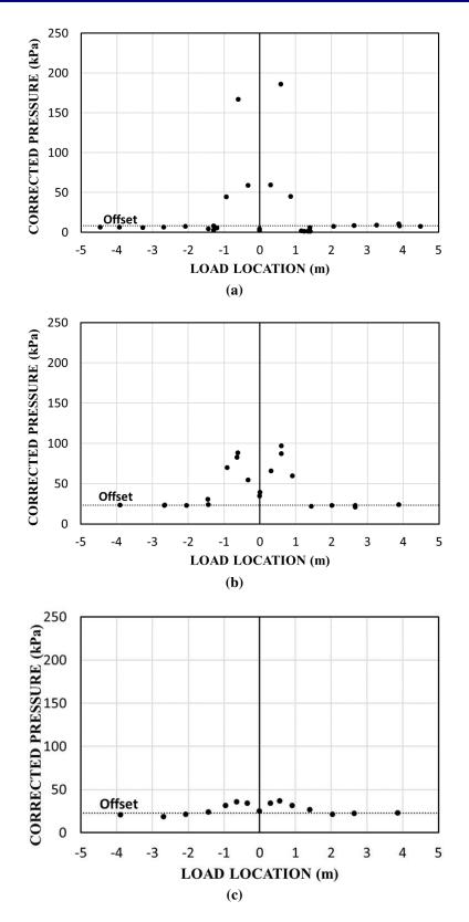
Figure 7. Pressure on top of the culvert for different heights of cover as the truck passes: a) 0.2 m of cover, b) 0.61 m of cover, c) 1.22 m of cover (after James et al., 1986).
