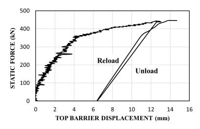
Figure 36. Static horizontal load-displacement curve for the barrier.
