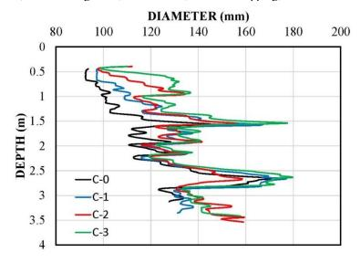
Figure 40. Borehole Erosion Test results (Briaud et al., 2015).
