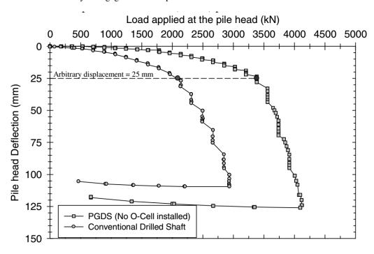
Figure 28. Load settlement curve for conventional and post grouted drilled shaft (King et al. 2015).
