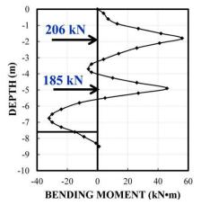
Figure 19. Wall bending moment profile at end of construction for two rows of anchors (after Chung, Briaud, 1992).
