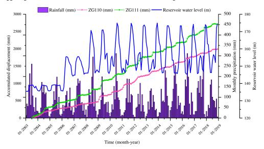
Figure 7. The accumulated displacement, rainfall, and reservoir water level at Bazimen landslide.
