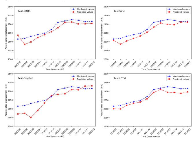
Figure 12. Predicted and monitored accumulated displacements at ZG111 with the MARS, SVM, LSTM, and Prophet
