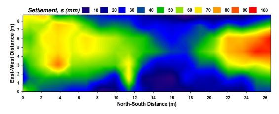
Figure 7. Spatially-distributed post-liquefaction settlements measured at Hollywood, SC and interpolated using ordinary kriging (Case A-1; data from Gianella and Stuedlein 2017).
