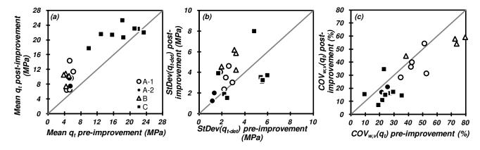
Figure 4. Comparison of pre- and post-installation: (a) mean  $q_t$ , (b) standard deviation in detrended  $q_t$ ,  $q_{t-deb}$  and (c) coefficient of inherent variability,  $COV_{w,v}(q_t)$ .
