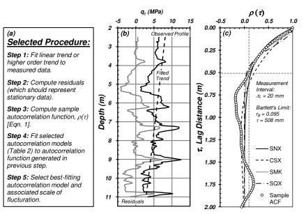
Figure 2. Demonstration of the procedure used to determine the scale of fluctuation for CPT P3-1 (Case A-1): (a) procedure steps; (b) observed and detrended q<sub>i</sub>; and (c) corresponding sample ACF and fitted autocorrelation models.
