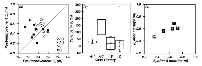
Figure 5. Evaluation of densification on the scale of fluctuation: (a) comparison of pre- and post-installation  $\delta_v$ , (b) range in change of  $\delta_v$ , and (c) effect of time on  $\delta_v$  for Zones 1 through 5B for Case A-1 (see Table 1).
