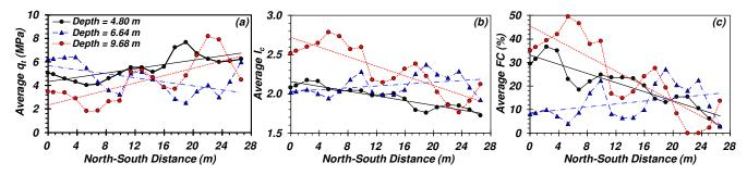
Figure 9. Representative horizontal profiles and fitted trends of (a)  $q_t$ , (b)  $I_c$ , and (c) FC averaged over the depths of 2.5 to 11 m for the E-W section offset of 4.56 m.
