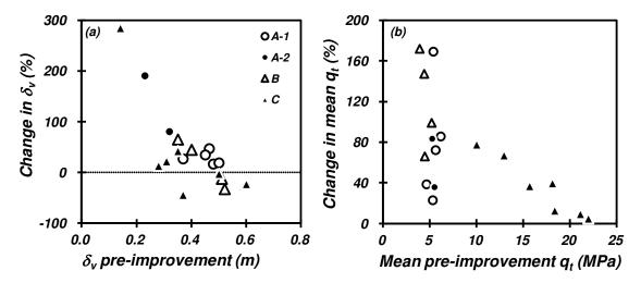
Figure 6. Post-treatment changes in: (a)  $\delta_v$  as a function of the initial autocorrelation, and (b) mean  $q_t$  as a function of initial mean  $q_t$ .
