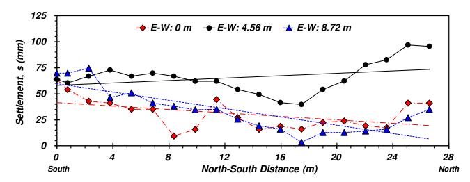
Figure 8. Representative horizontal profiles and fitted trends in the measured post-liquefaction settlement.
