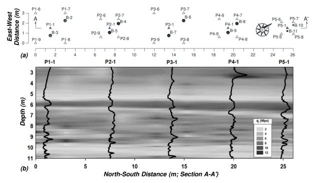
Figure 1. Site and subsurface conditions at the Hollywood, SC test site (Case A-1) including: (a) exploration plan for Zones 1-5, and (b) pre-treatment CPT cone tip resistance measured within the liquefiable layers along Section A-A' and corresponding spatial variation inferred from geostatistical analyses reported by Bong and Stuedlein (2017; 2018).
