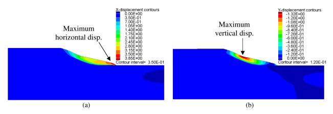
Figure 16. Displacement contours of the slope at general failure: (a) horizontal displacement and (b) vertical displacement. (Note: x-displacement is horizontal displacement, and y-displacement is vertical displacement. Unit of the contour plots is in meters.)
