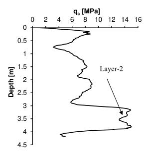
Figure 7. Cone tip resistance versus depth.
