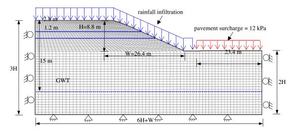
Figure 10. Model setup: geometry, grid discretization, boundary, and internal conditions.
