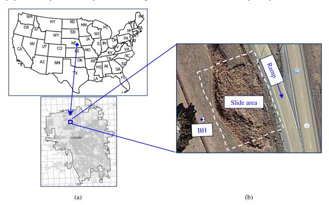
Figure 1. (a) Location of the failed slope site, and (b) plan view of the slope (2020) (note: BH is to mean borehole).
