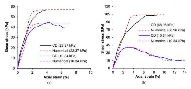
Figure 12. Numerical calibration of the CD test results: (a) Layer-1 and (b) Layer-3.
