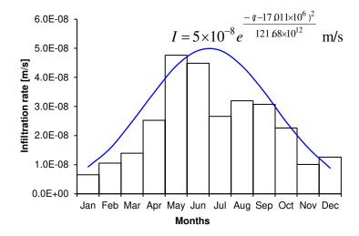
Figure 11. Average rainfall intensity and infiltration rate model (average of 20 years data).
