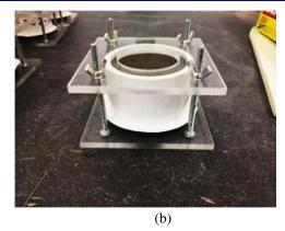
Figure 8. (a) Compaction mold, and (b) specimen enclosed in PVC molds before weathering.
