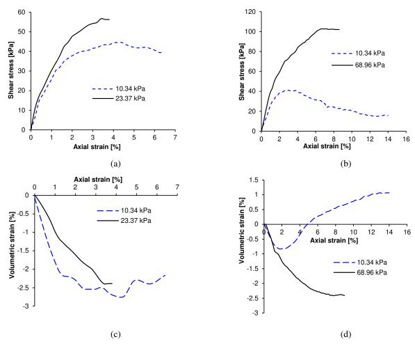
Figure 6. Isotopically consolidated drained triaxial test results: (a) shear stress vs. axial strain for Layer-1, (b) shear stress vs. axial strain for Layer-3, (c) volumetric strain vs. axial strain for Layer-1, and (d) volumetric strain vs. axial strain for Layer-3 (note: numbers in the legends are confining stresses used).
