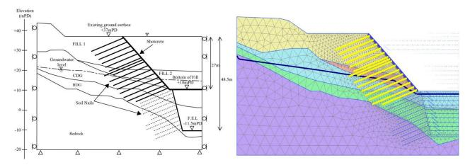
Figure 22. Finite element model for HMT Site formation.
