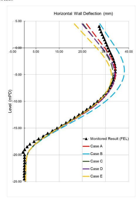
Figure 16. Horizontal wall deflection profiles of the HS models for sensitivity study plotted with inclinometer data at GL 50 seaward side.
