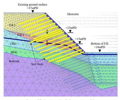
Figure 27. Position of soil elements A and B.
