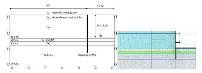
Figure 13. Finite element model for GL 50 at seaward side (FEL = Final Excavation Level).
