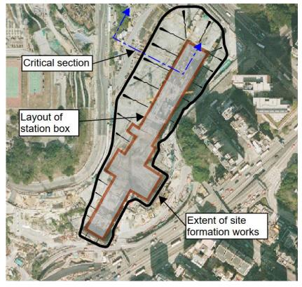
Figure 18. General view of the HMT excavation works.
