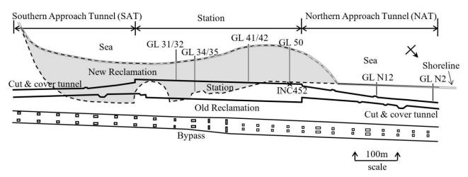
Figure 6. Layout plan of the Tsuen Wan West project (after Pickles et al, 2006); GL = grid line.
