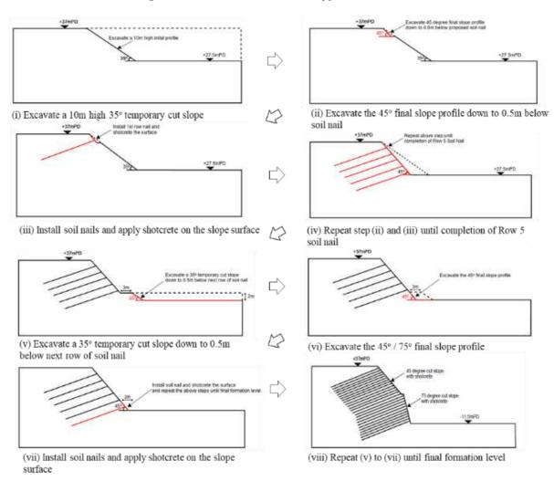
Figure 21. Construction Sequence of HMT site formation works.
