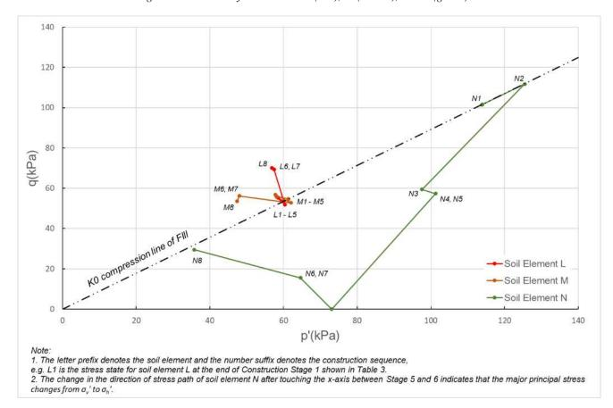
Figure 30. Stress paths from initial stage to final stage for soil element L (red), M (brown), and N (green).
