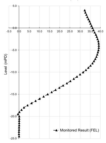
Figure 11. Wall deflection at GL50 seaward side at final excavation stage (after Pickles et al, 2003).
