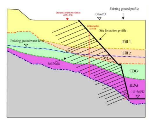
Figure 19. Cross-section of the HMT Station site.
