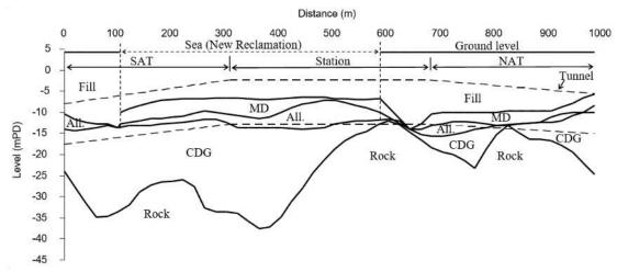
Figure 7. Geological profiles of Tsuen Wan West Station along the seaward side diaphragm wall before New Reclamation (after Pickles et al, 2006); All. = alluvium; MD = marine deposits; CDG = completely decomposed granite.
