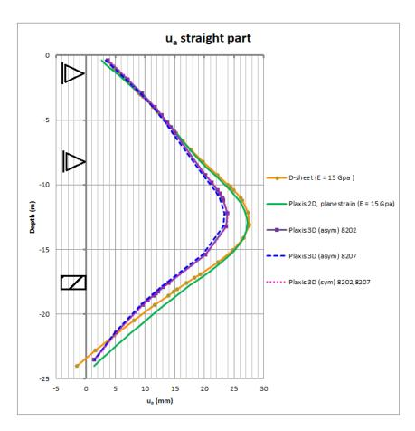
Figure 6. Displacements calculated for the straight walls.
