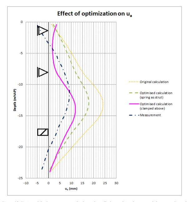
Figure 15. Horizontal displacements perpendicular to the wall after applying the proposed changes to the model.
