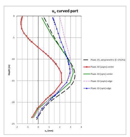
Figure 7. Displacements in the axisymmetric and transition zones.
