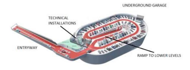
Figure 1. Three-dimensional view of the parking garage underneath the Garenmarkt.
