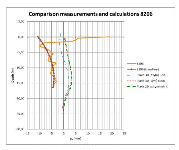
Figure 13. Comparison of the measured and calculated displacements near the center of the curved part of the excavation.
