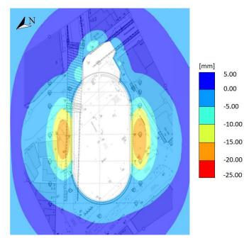
Figure 8. Calculated settlements from the asymmetric PLAXIS 3D model.
