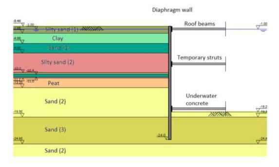
Figure 3: Cross-section of the excavation.
