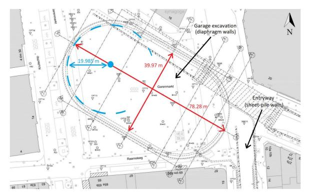
Figure 2. Dimensions of the excavation.
