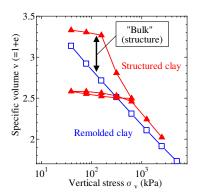
Figure A1. Typical oedmeter test results on structured clay and remolded clay (Noda et al., 2005).
