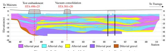
Figure 1. Soil strata in the Mukasa area (longitudinal section).
