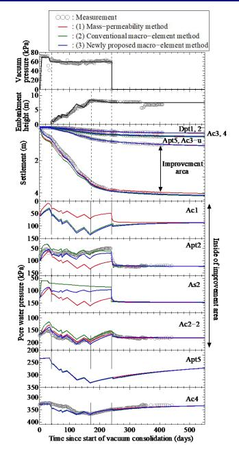
(a) Time-settlement / pore water pressures relations at the center of embankment
