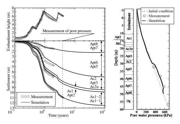
Figure 6. Simulation and predictions of large-scale settlement of the test embankment (STA 498+25, Tashiro et al., 2015).
