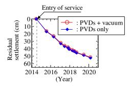
Figure 12. Comparison of residual settlement (measurements).
