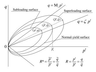
Figure A2. Three loading surfaces.
