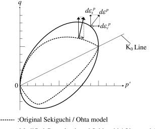
:Modified Cam-clay-based Sekiguchi / Ohta model
