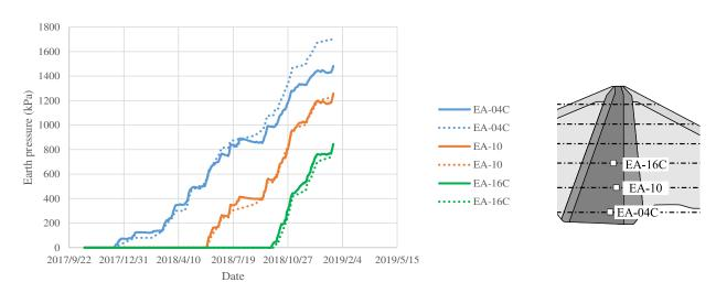
Figure 18. Time histories of earth pressure (downstream core zone).
