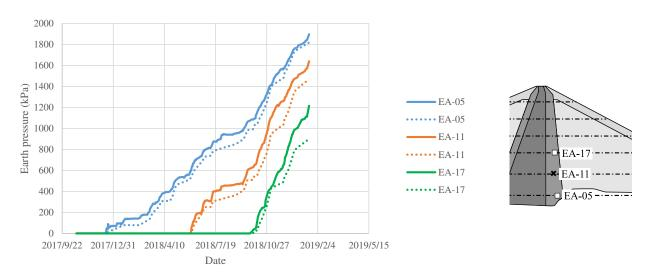
Figure 19. Time histories of earth pressure (downstream filter zone).
