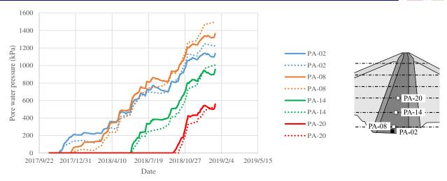
Figure 11. Time histories of pore water pressure (center core zone).
