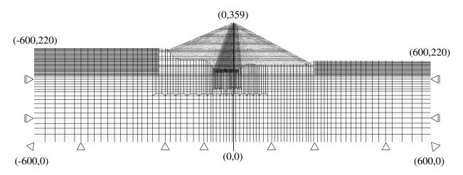
Figure 2. Finite element mesh of foundation and dam body (Unit: m).
