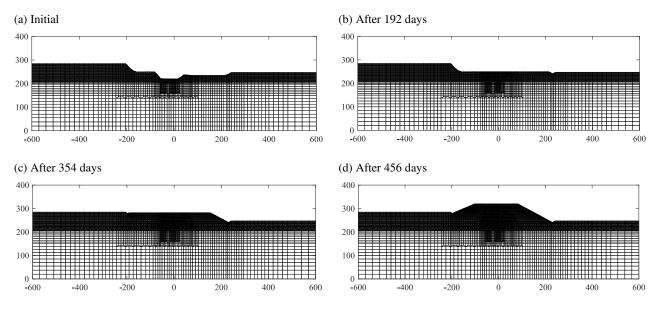
Figure 4. Cross sections of dam during construction (Unit: m).
