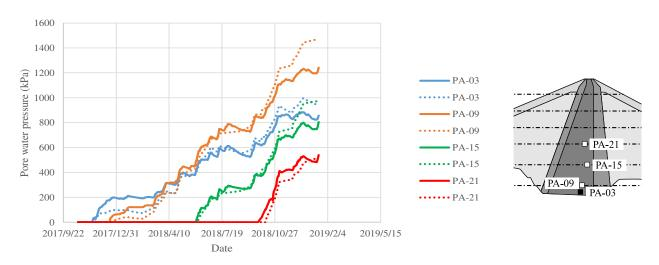
Figure 12. Time histories of pore water pressure (downstream core zone).
