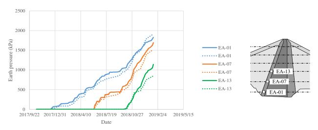
Figure 15. Time histories of earth pressure (upstream filter zone).
