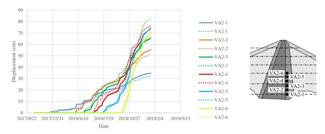
Figure 6. Time histories of displacement (filter zone).
