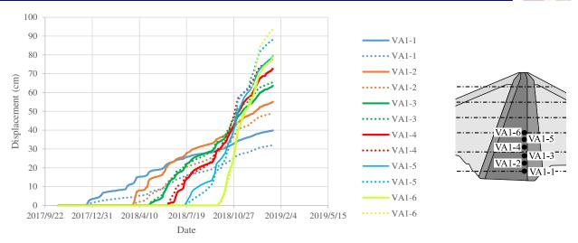
Figure 5. Time histories of displacement (core zone).
