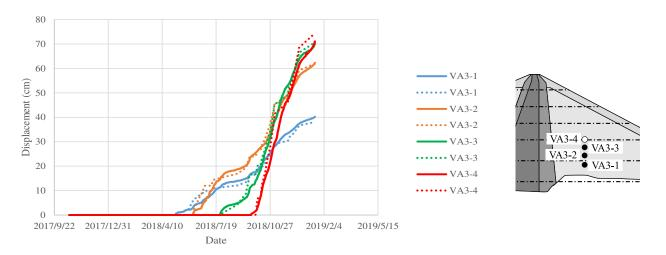
Figure 7. Time histories of displacement (downstream rock zone).
