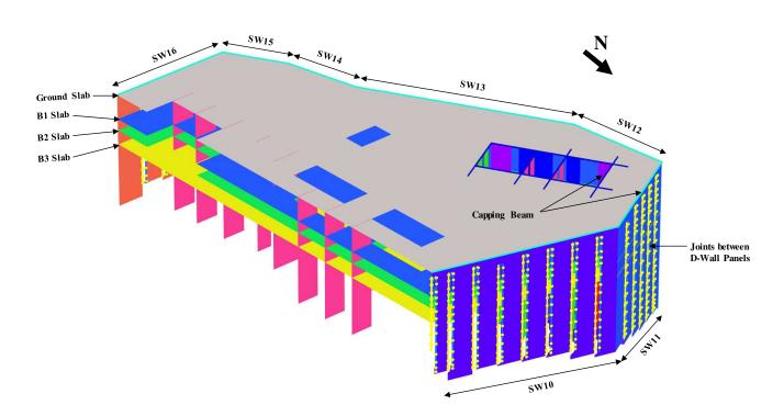
Figure 8. Schematic view of the PLAXIS 3D model.
