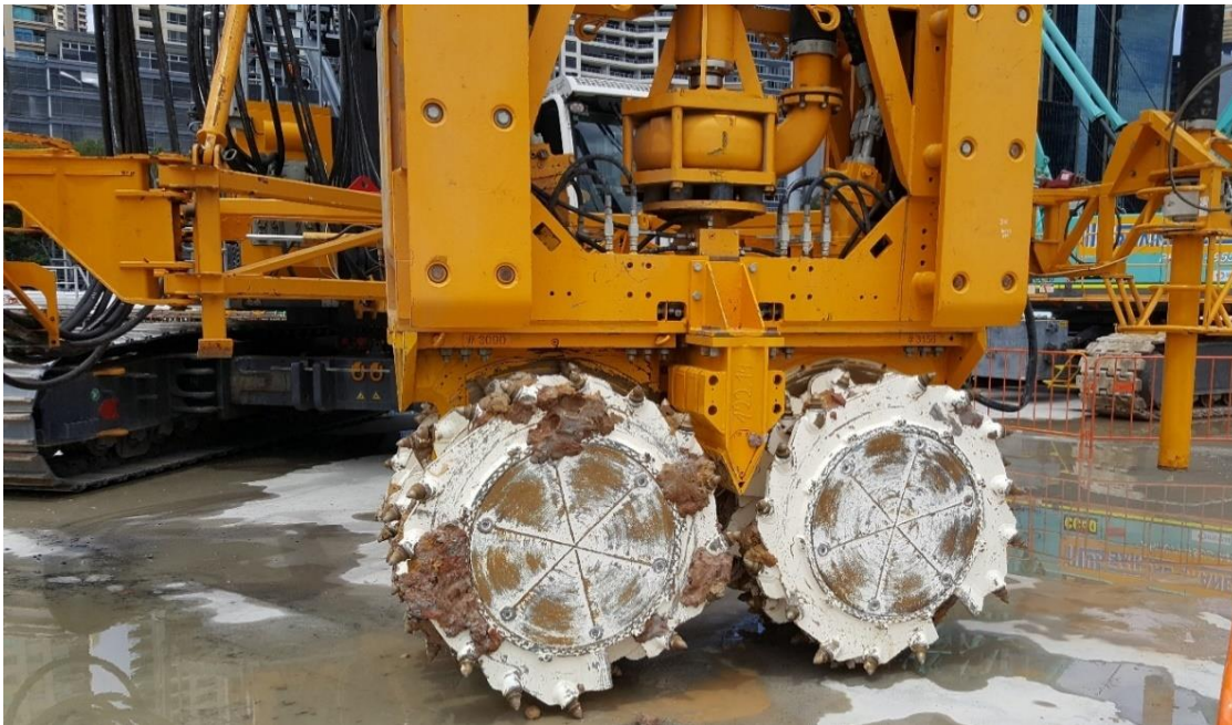
Figure 14. Hydraulic cutter with protruding teeth.
