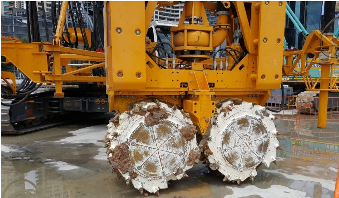
Figure 14. Hydraulic cutter with protruding teeth.
