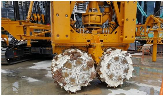
Figure 14. Hydraulic cutter with protruding teeth.
