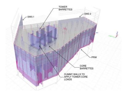
Figure 10. Snapshot of structural model.
