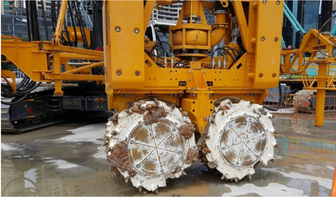
Figure 14. Hydraulic cutter with protruding teeth.
