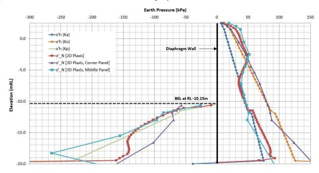
Figure 11. Typical lateral earth pressure diagram for a D-Wall.
