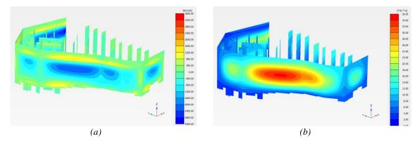
Figure 12. Example of PLAXIS 3D contour maps: (a) Out-of-plane bending moments and (b) Out-of-plane total displacements.
