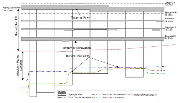
Figure 6. A typical section of the ground profile at Site location – Section B-B.
