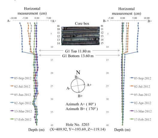
Figure 15. Surface and subsurface displacements measured by I203.
