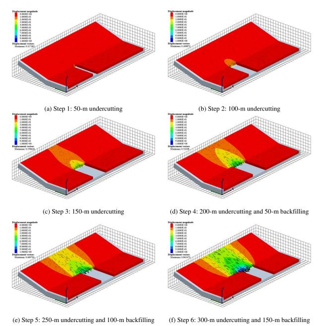
Figure 8. Total displacement contour and vectors of simple Area 4.1 undercut slope model.
