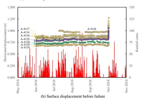
Figure 30 Surface displacement of 2<sup>nd</sup> Stage of Area 4.1.
