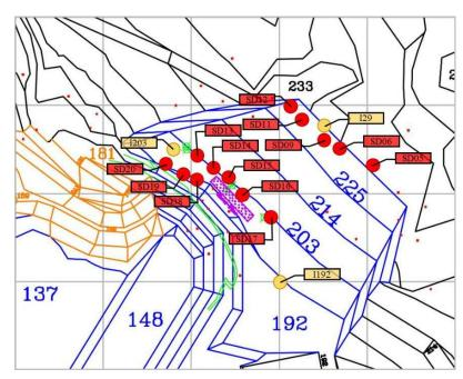
*Figure 14. Locations of prisms and inclinometers in Area 4.1.*
