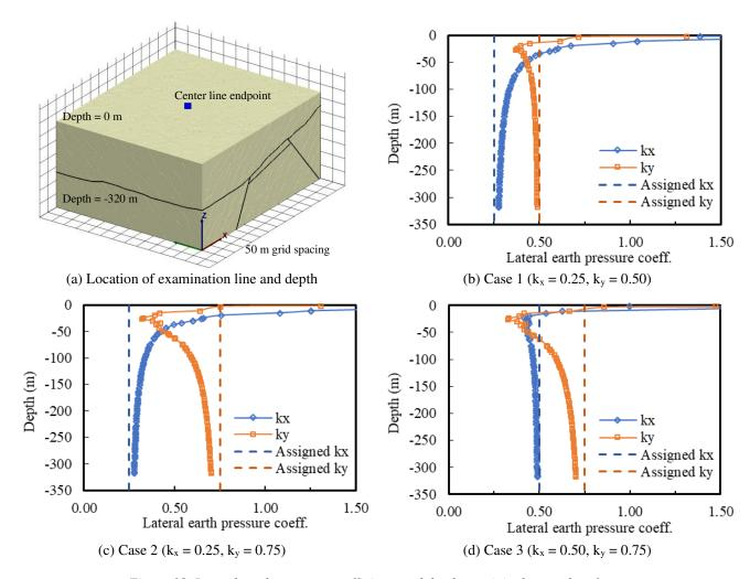
Figure 18. Lateral earth pressure coefficients and depth at original ground surface.
