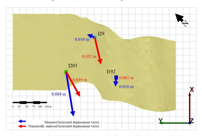
Figure 26. Subsurface displacements of inclinometer at G1 interface.
