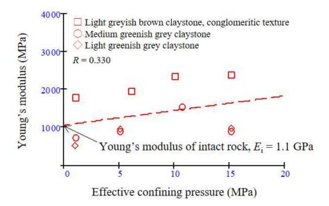
Figure 5. Elastic moduli and applied confining pressures.
