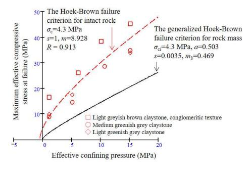
Figure 4. Principal stresses at failure for all samples.
