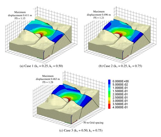
Figure 20. Maximum total displacements of undercut models.
