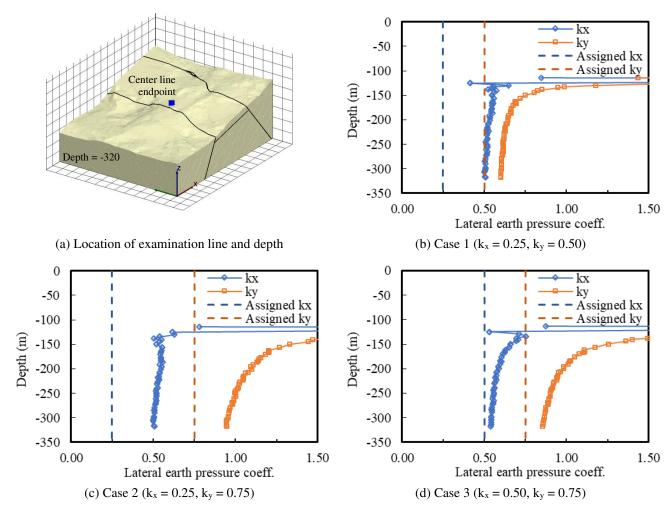
Figure 19. Increase in lateral earth pressure coefficients and depth at ground surface 2011.
