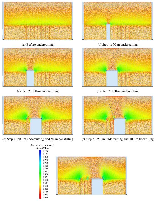
(g) Step 6: 300-m undercutting and 150-m backfilling
