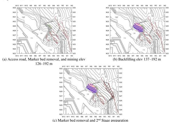
Figure 11. Sequential excavation of the 1<sup>st</sup> Stage in Area 4.1.
