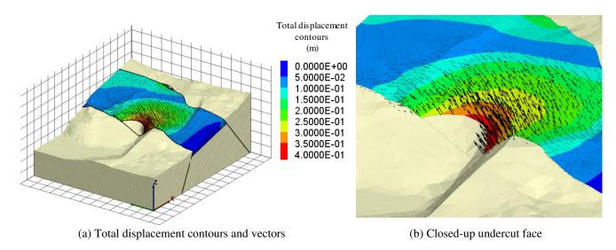
Figure 22. Total displacement contours and vectors of undercut model.
