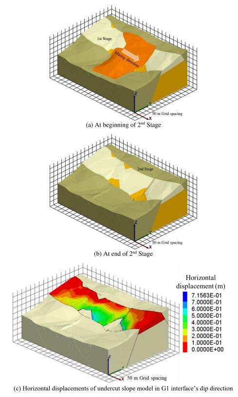
Figure 27. 2<sup>nd</sup> Stage numerical model and its horizontal displacements of undercut.
