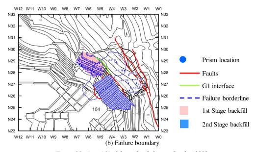
Figure 29. Area 4.1's debris after failure in October 2018.
