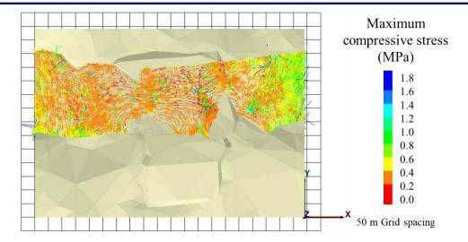
Figure 28. Principal stress trajectories in potential sliding block of 2<sup>nd</sup> Stage.
