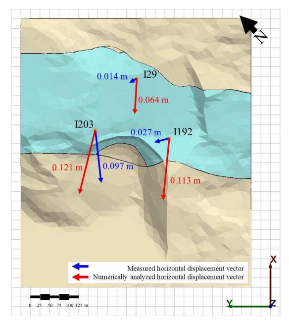
Figure 25. Horizontal displacements of inclinometer collars.
