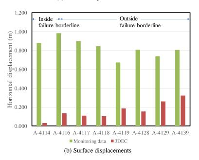
Figure 31 Comparison of surface displacements at 2<sup>nd</sup> Stage of Area 4.1.
