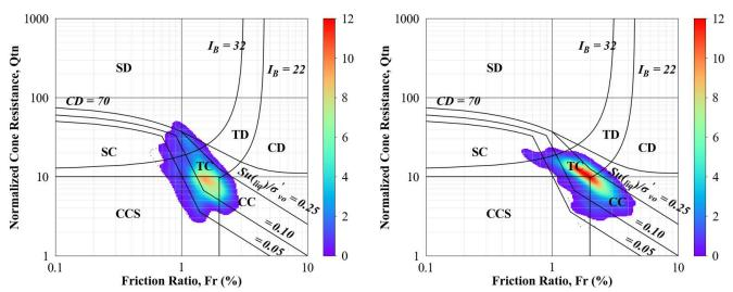
Figure 16. SBTn plots for Test Pad 1 with contours of  $Su_{(min)}/\sigma'_{vo}$  before (left) and after (right) Test Pad loading (for saturated tailings above EL. 763 m).
