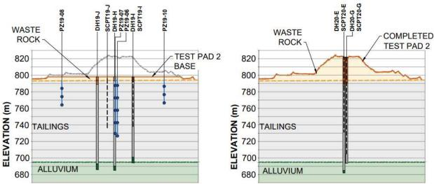
Figure 10. Tailings site investigations at Test Pad 2 before (left) and after (right) pad construction.
