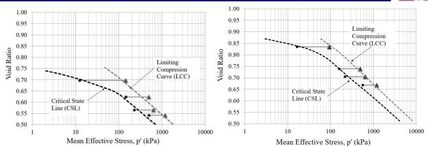
Figure 21. Curved CSLs for Coarse (left) and Fine (right) laboratory tailings samples.
