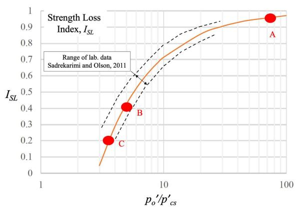
Figure 4. Strength Loss Index (I<sub>SL</sub>) versus Reference Stress Ratio (p'<sub>o</sub>/p'<sub>cs</sub>) for a range of sands with three tests on Erksak sand added in red.
