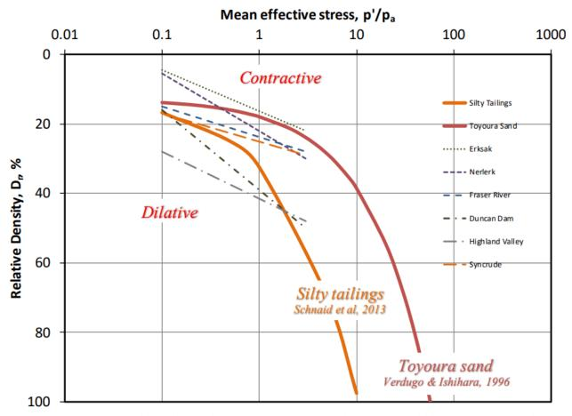
Figure 1. Comparison of published Critical State Lines (CSL) for a wide range of sand-like soils ( $p_a$  = atmospheric pressure ~ 100kPa).
