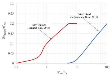
Figure 5. Variation of  $Su_{(min)}/\sigma'_{vo}$  from triaxial compression tests as a function of normalized effective confining stress  $(\sigma'_{vo}/p_a)$  for Erksak sand (Jefferies and Been, 2016) and a silty (gold) tailings (Schnaid et al., 2013).
