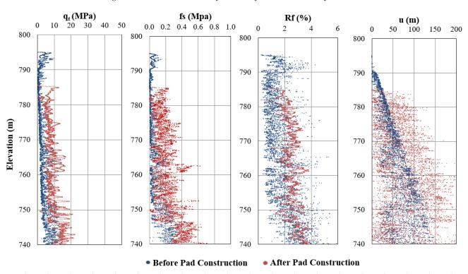
Figure 13. Raw SCPT data before and after construction of Test Pad 2.
