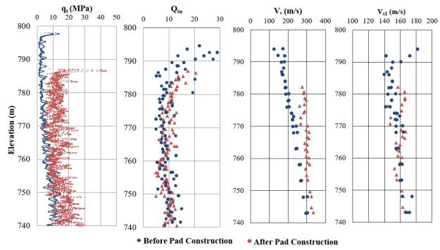
Figure 14. SCPT data before and after construction of Test Pad 1.
