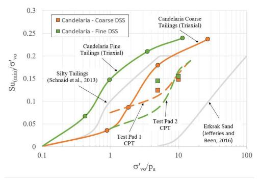
Figure 22. Variation of  $Su_{(min)}/\sigma'_{vo}$  for Candelaria tailings as a function of normalized effective confining stress ( $\sigma'_{vo}/p_a$ ), (with reference to Erksak sand and Schnaid silty tailings).
