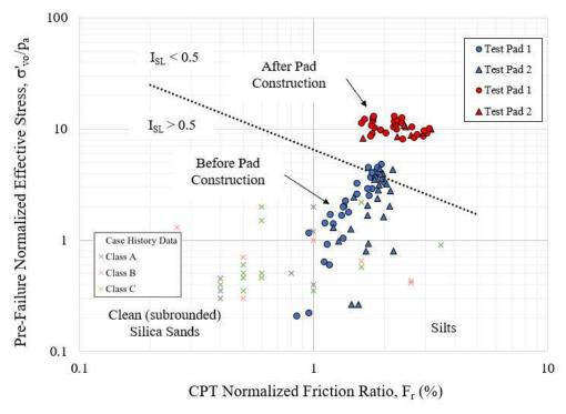
Figure 23. Variation in large strain undrained behavior as a function of CPT normalized friction ratio (Fr) (modified from Robertson, 2017, case history data from Robertson, 2010).
