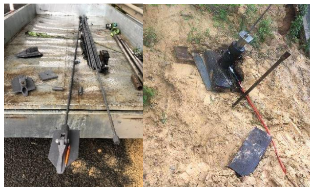
Figure 5. Percussion anchor (180-millimeter head) and load testing.
