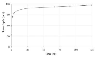
Figure 15. Scour depth progress of Set L.2, Source: FHWA.
