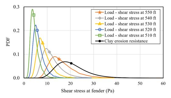
Figure 22. Bed shear stress distribution for total fender scour, Source: FHWA.
