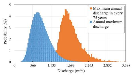
Figure 21. PMF of annual maximum discharge and maximum annual discharge in every 75 years for the Lafayette Avenue Bridge, Source: FHWA.
