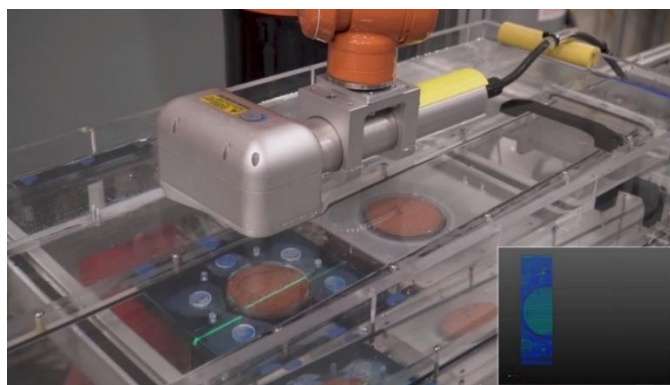
Figure 8. Laser scanner scanned soil surface and digitized soil surface (inset), Source: FHWA.
