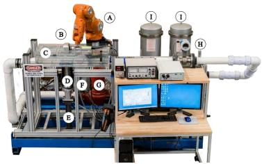
$A = Robotic \ arm; \ B = laser \ scanner; \ C = flow \ channel; \ D = 3-in \ Shelby \ tube \ soil; \ E = hydraulic \ piston; \ F = shear \ sensor; \ G = flow \ pump; \ H = flow \ meter; \ and \ I = filter \ cylinder.$
