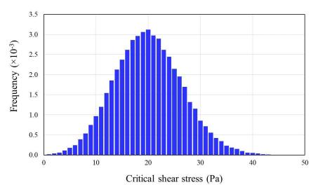
Figure 12. Histogram of the 50,000 critical shear stresses, Source: FHWA.
