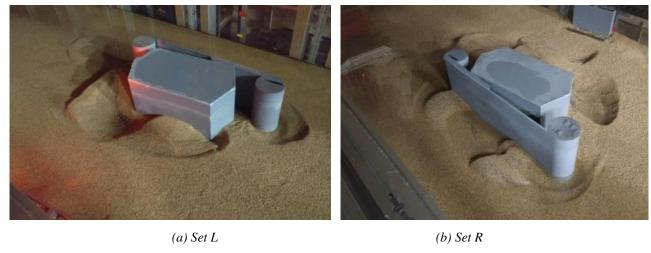
Figure 16. Final scour hole around the pier and fender, Source: FHWA.
