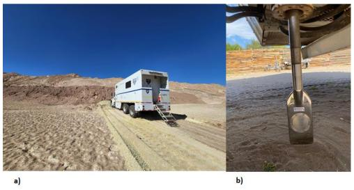
Figure 3. In-situ testing: a) CPT truck, b) DMT probe.
