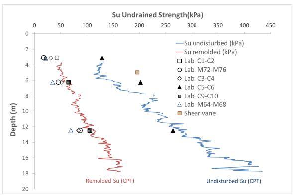
Figure 7. Comparison between S<sub>u</sub> values obtained from CPT and laboratory triaxial tests.
