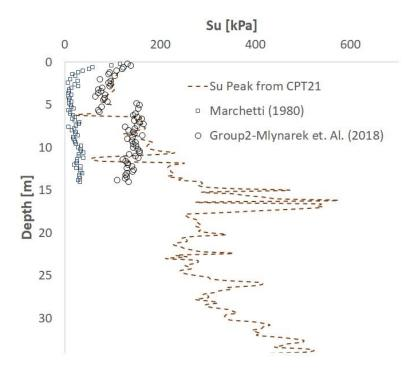
Figure 8. Comparison between S<sub>u</sub> values obtained from CPT and DMT tests at CPT21.
