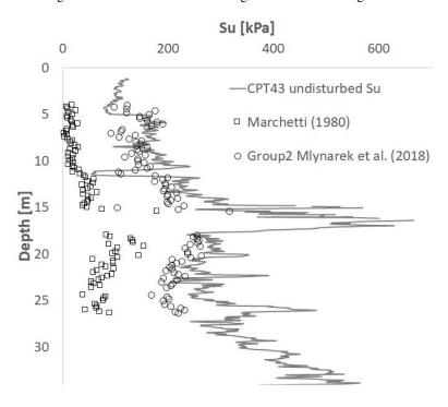
Figure 9. Comparison between S<sub>u</sub> values obtained from CPT and DMNT tests at CPT43.
