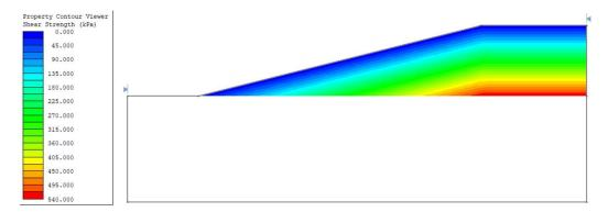
Figure 12. Deduced shear strength using SHANSEP.
