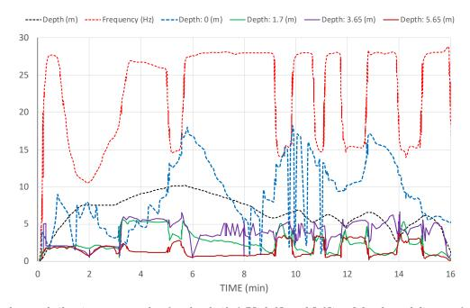
b) Horizontal ground vibrations measured at four levels (0, 1.75, 3.65, and 5.65) at 8.9 m lateral distance from the probe. Figure 10. Horizontal ground vibrations (RMS) on, and at three levels below the ground surface, at 3.1 and 8.9 m distances from the center of the compaction probe.
