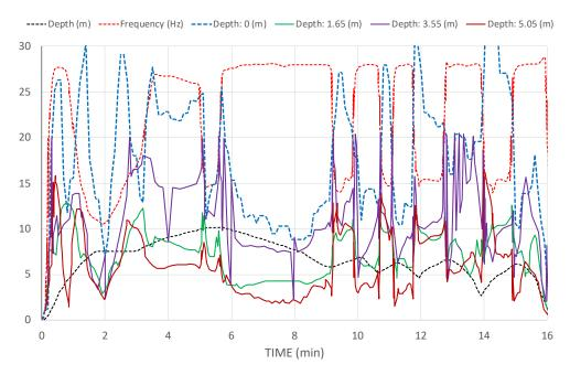
a) Horizontal ground vibrations measured at four levels (0, 1.65, 3.55, and 5.05) at 3.1 m lateral distance from the probe.
