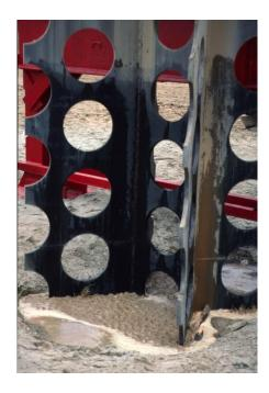
a) Triaxial geophone located at 6 m distance from the compaction probe. b) Liquefaction during DVVCr.
