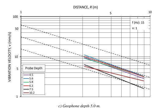
Figure 11. Attenuation of horizontal vibration velocities during resonance compaction.
