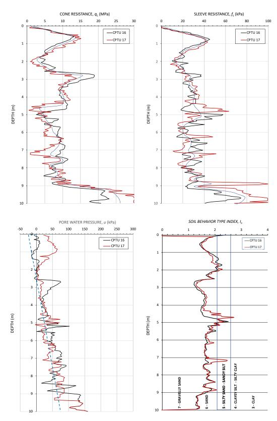
Figure 3. CPTU results prior to compaction (CPTU 16 and 17).
