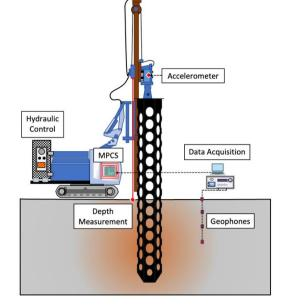
a) Vibrator clamped to flexible compaction probe.
