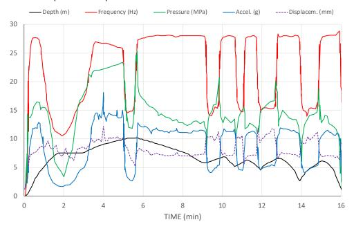
Figure 7. Performance data of the compaction machine.
