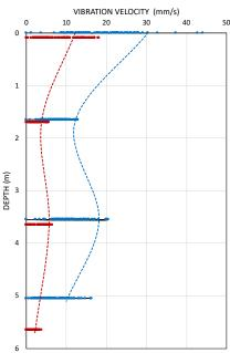
Figure 12. Variation of horizontal ground vibration velocity (RMS) at 3.1 (blue) and 8.9 m (brown) as a function of depth during probe penetration to 10 m depth.
