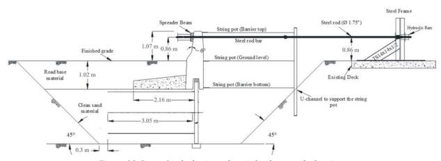
Figure 16. Set up for the horizontal static load test on the barrier.
