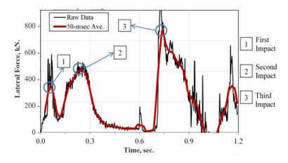
Figure 3. Horizontal impact force as a function of time in FEM simulation.
