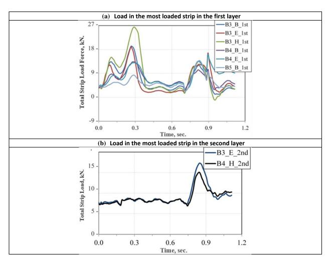
Figure 6. Total load in the most loaded strip for the first and second rows of strips in FEM simulation: (a) load in the most loaded strip in the first layer, and (b) load in the most loaded strip in the second layer.
