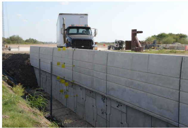
Figure 12. Test set up just before impact test.
