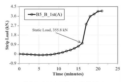
Static Load Rate in the Barrier, 22.24 kN/min Figure 18. Load in top strip below barrier loading point.
