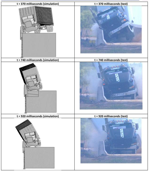
Figure 14. Comparison between simulation and test of sequential views of the impact.
