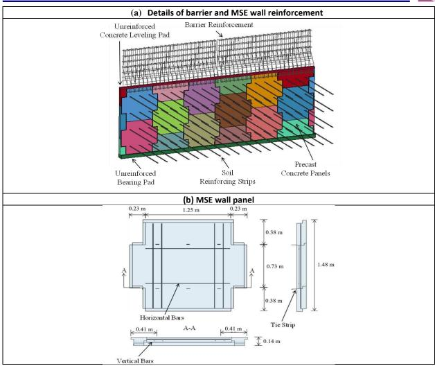
Figure 2. Barrier-moment slab and MSE wall model: (a) details of barrier and MSE wall reinforcement, and (b) MSE wall panel.
