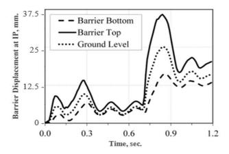
Figure 4. Barrier displacement during impact in FEM simulation.
