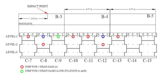
Figure 11. Location of the instrumented reinforcing strips.
