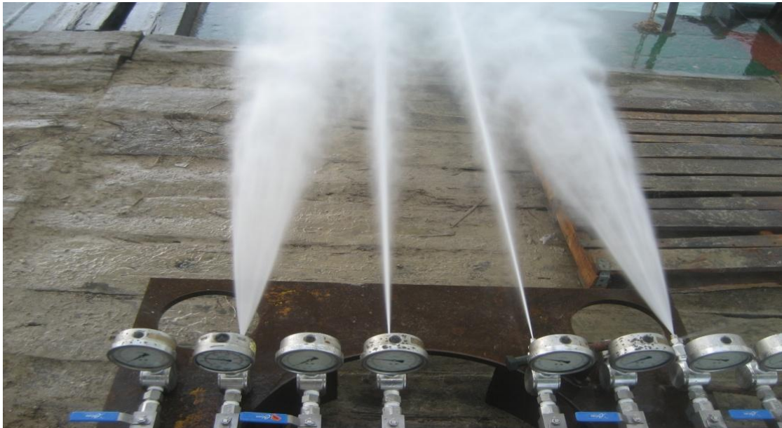
Figure 11. Testing of Nozzles: The two nozzles at the sides are spreading the water at an angle of 25°, and the two in the middle are jetting it linearly.
