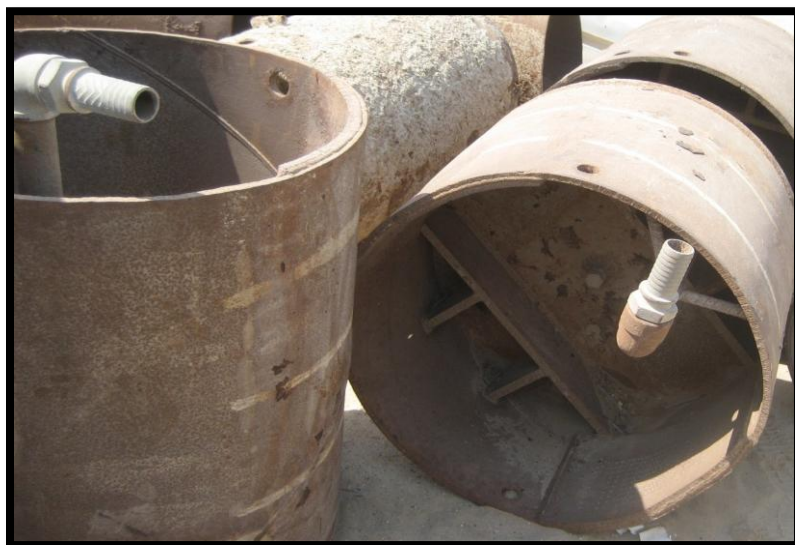
Figure 5. Uplift Water Pressure Method setup, showing pile cap plugs with a 90° elbow and nipple.
