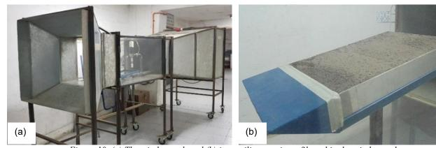
Figure 10. (a) The wind tunnel, and (b) iron tailing specimen filtered in the wind tunnel.
