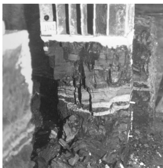
Figure 9. Failed block of coal after testing (Hudek, 1986).
