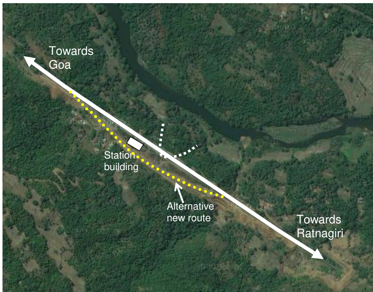
Figure 1. Nivsar Station in Ratnagiri District of Maharashtra (Source: Google earth). Note: The dashed line shows the approximate location of the embankment failure .
