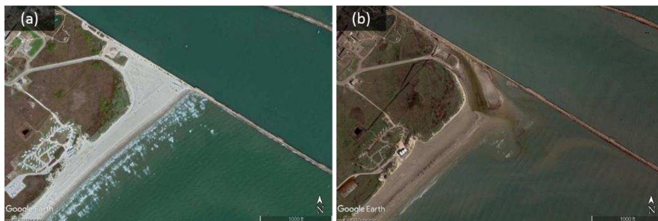
Figure 3. (a) Pre-storm satellite imagery (imagery date February 22, 2017) and (b) post-storm satellite imagery (imagery date August 29, 2017) show the eroded runnel created during Hurricane Harvey near Port Aransas Pass (location 27^{\circ}50'6.39''\text{N} , 97^{\circ}2'50.56''\text{W} ). Map data: Google Earth, Digital Globe.
