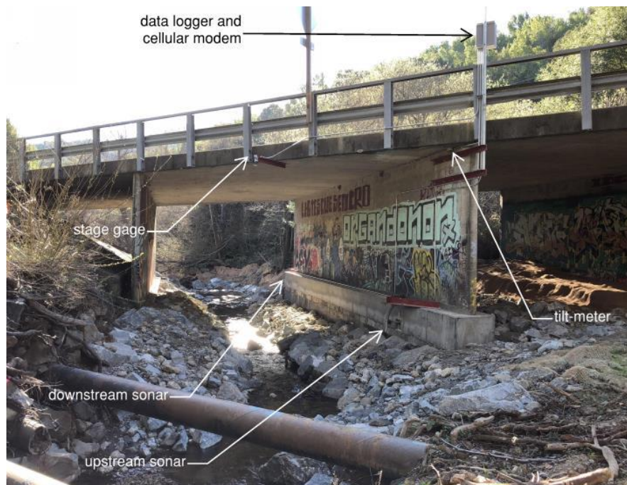
Figure 11. Looking downstream at Piers 3 and 4 (after monitoring device installation, February 2018).
